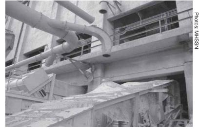
Report by international commission organized by Maquiladora Health & Safety Support Network documented how dust collectors have been disconnected by the company (above), leading to huge accumulations of deadly silica dust as well as dangerous holes in the floor.
