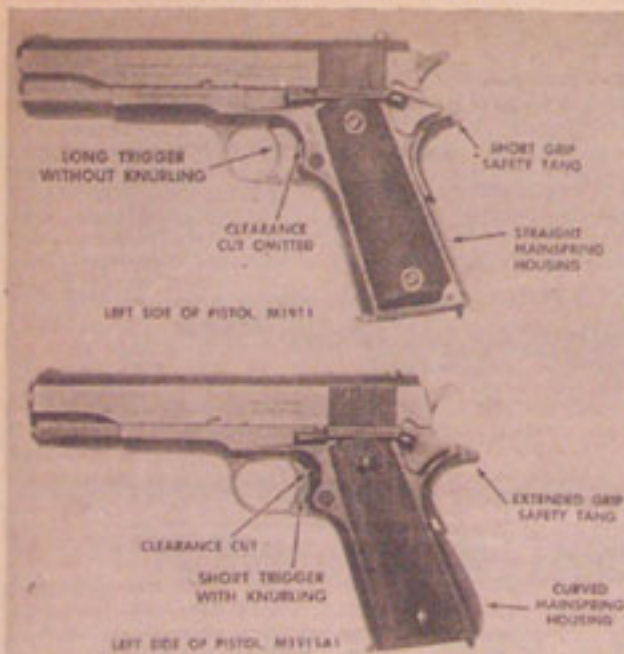
Pistols, Automatic, Caliber .45 M1911 and M1911A1, showing differences between models.
