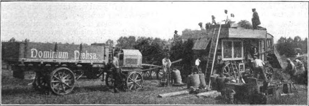
THE MOTOR OF A MOTOR WAGON DRIVING A THRESHING MACHINE.
