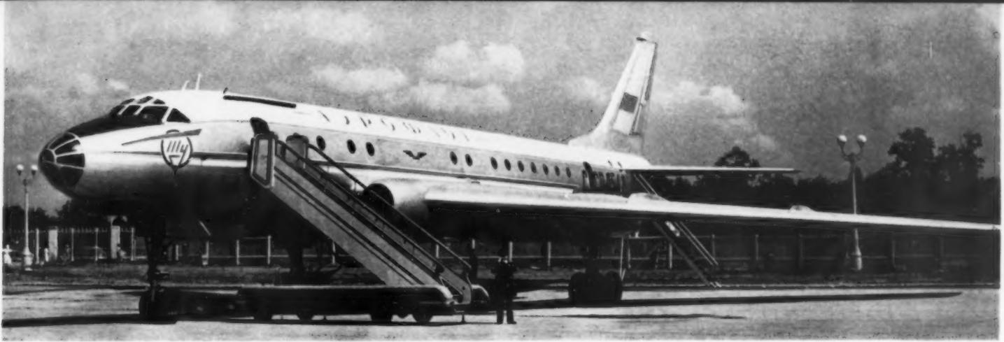
The TU-104A jet airliner carries seventy passengers and has a cruising speed of 550 miles per hour. It is one of several new types manufactured by Soviet industry for civil airlines. Among the new turbo-prop planes is an airliner that carries 200 passengers and cruises at 600 miles per hour.
