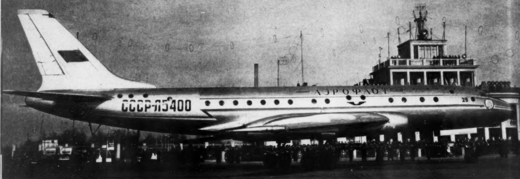
THE TWO-ENGINE TU-104, SEATING 50 PASSENGERS, WAS THE FIRST JET-POWERED AIRLINER TO BE USED FOR COMMERCIAL SERVICE. ITS DESIGNER IS ANDREI TUPOLEV.
