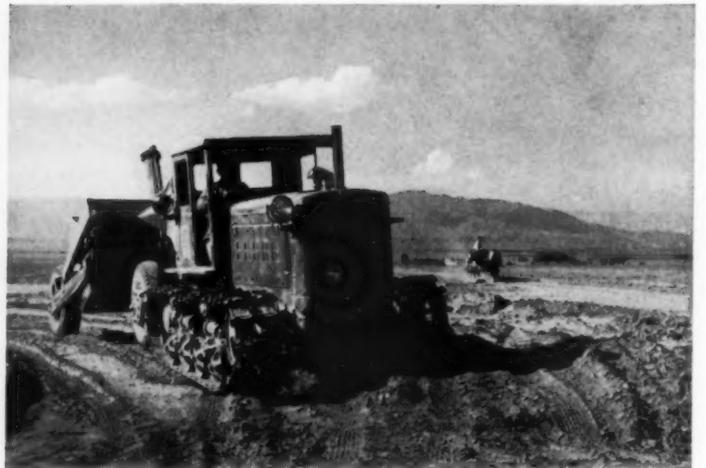
EARTH-LEVELING MACHINE USED TO PREPARE DRY STEPPELANDS FOR NEW CROPS.
