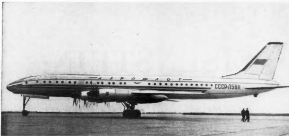
THE TU-114, A FOUR-ENGINE TURBOPROP, CAN FLY NON-STOP FROM MOSCOW TO NEW YORK IN 10-12 HOURS.
