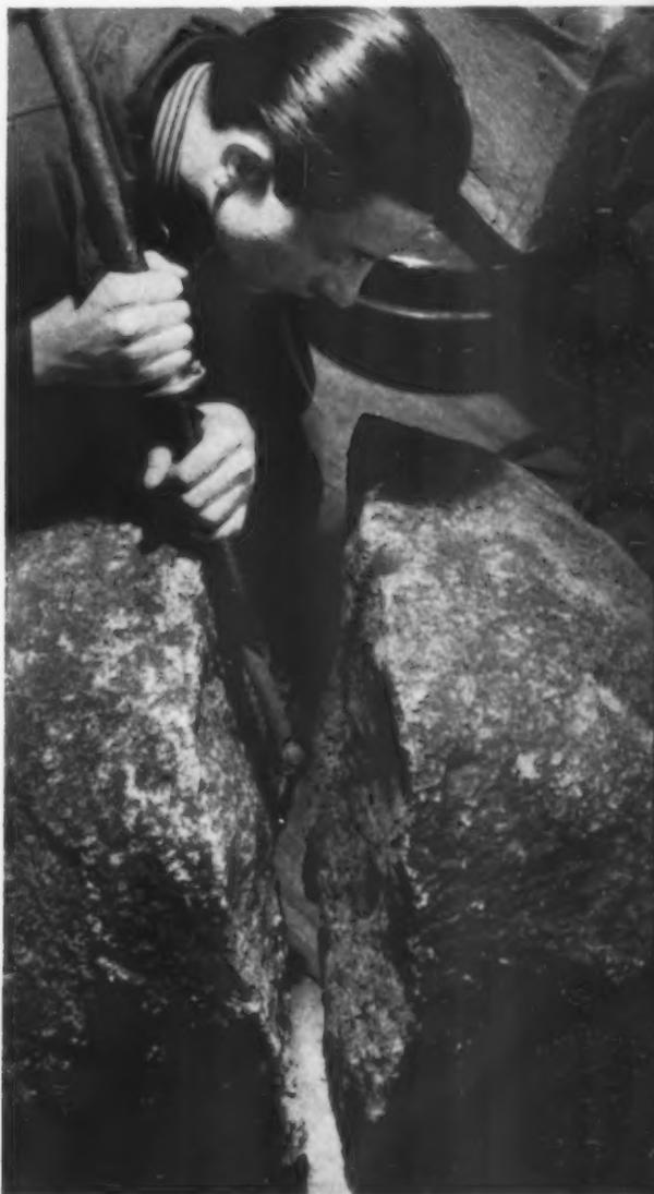
This discharger, designed by Lev Yutkin, splits a block of granite in a matter of a few seconds.
