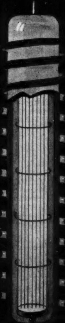
With a strong discharge current, the field tears the plasma off the walls, compresses and heats it. But without the coil, the column becomes unstable.
