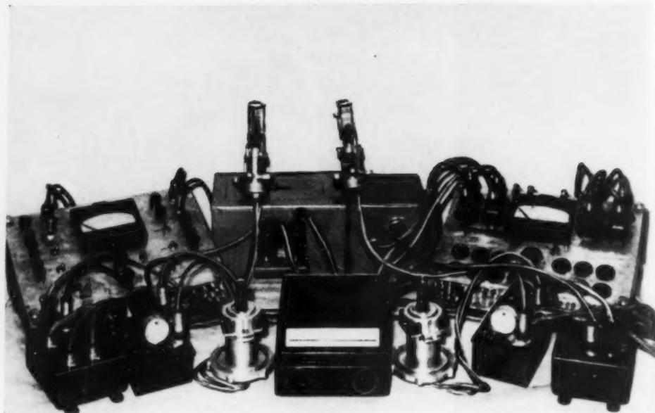
THESE IONIZATION AND MAGNETIC GAUGES ARE BEING TESTED PRIOR TO THEIR INSTALLATION ON ROCKETS.
