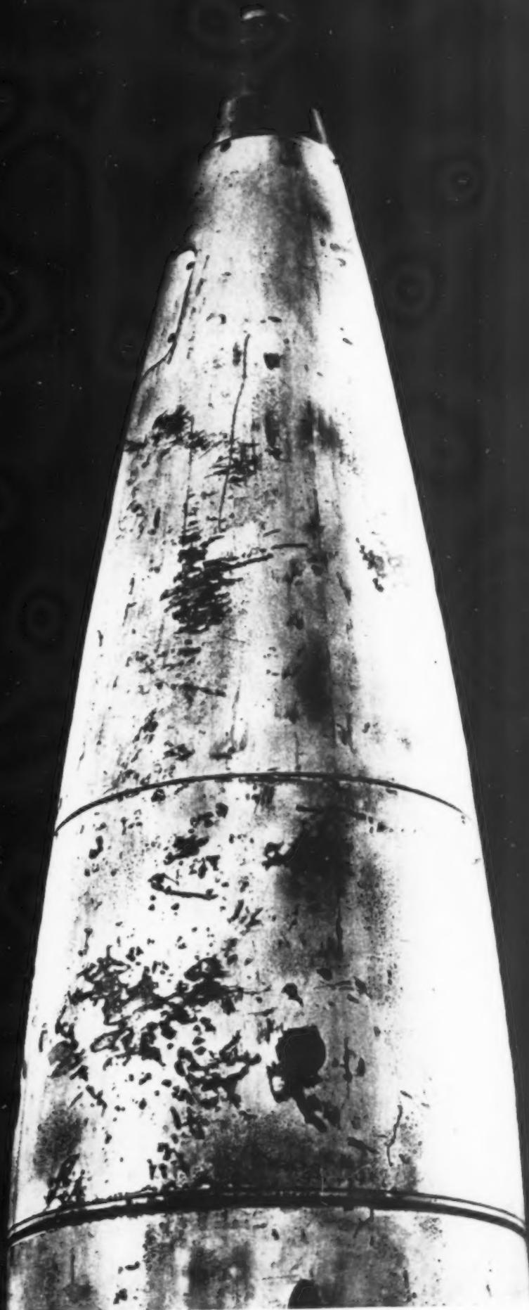
ROCKET CONE SCARRED BY METEOR PARTICLES DURING UPPER ATMOSPHERE TRIPS.
