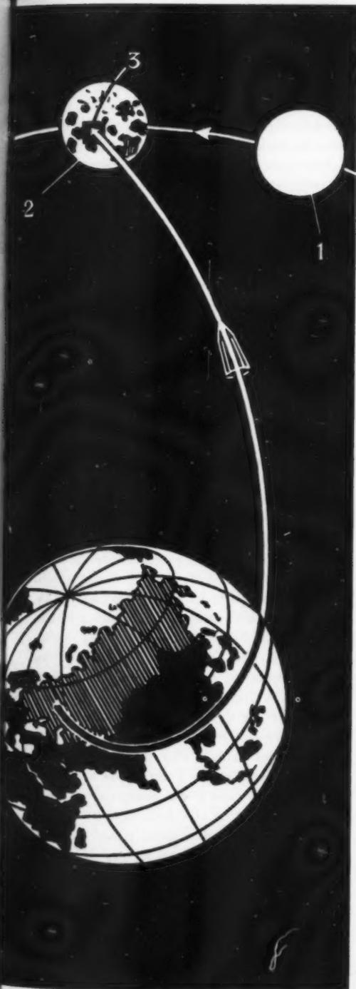
This chart shows the trajectory of the second Soviet cosmic rocket. 1—the position of the moon at zero hour; 2—the position of the moon at the time the rocket made impact; 3—the area of the moon where the rocket landed.
