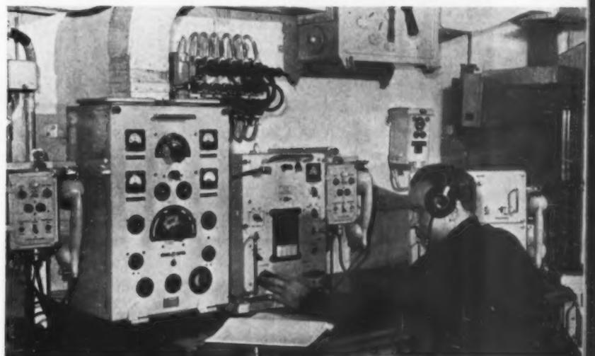
Radio receivers and transmitters keep the icebreaker in touch with shore, planes and other ships, and its own helicopter is used for reconnaissance.
