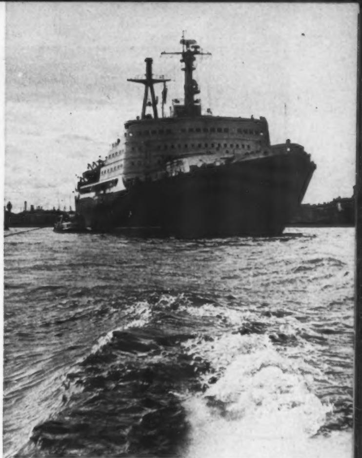
The 440-foot long, 92-foot wide, five-story high *Lenin* has a 16,000-ton displacement and a cruising speed of 18 knots.
