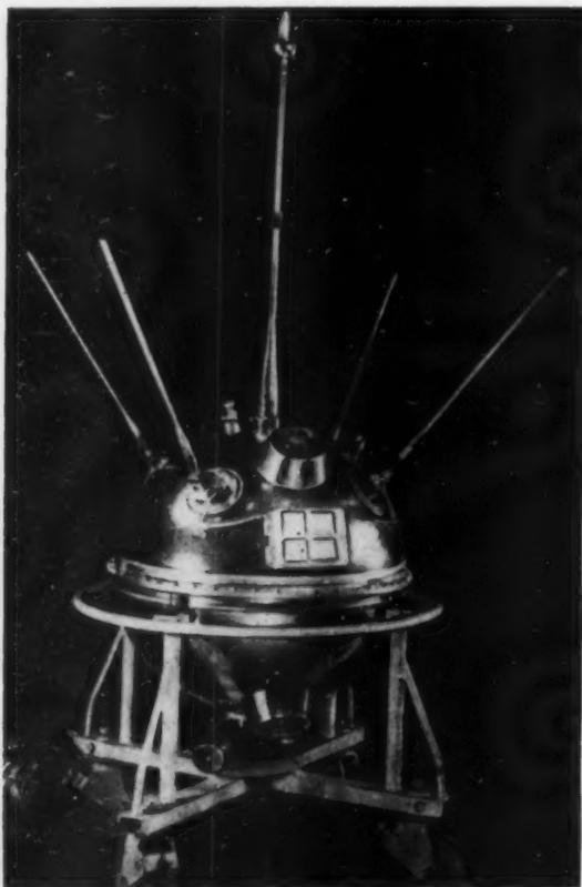
The instrument frame of the container with its equipment and power sources shown on an assembly carriage.
