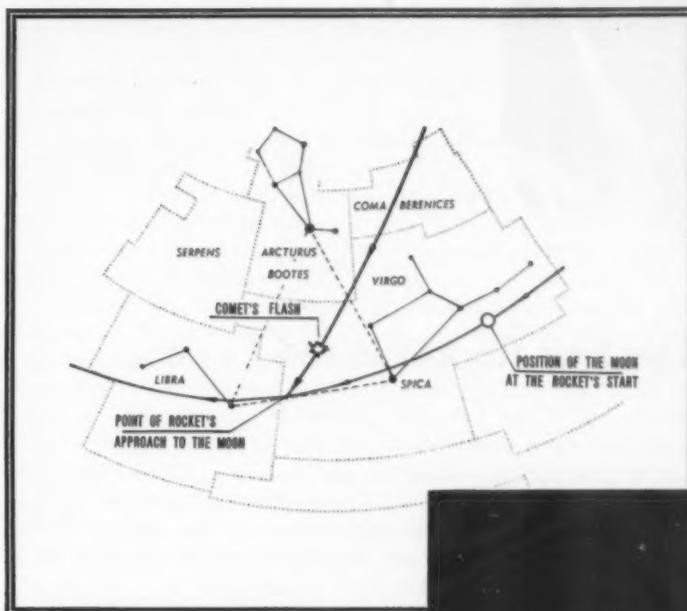
Constellation map shows the rocket's path toward the moon. At the right is an actual photograph of the flash of the artificial comet formed by the rocket on January 3 at the distance of 70,000 miles from the earth.
