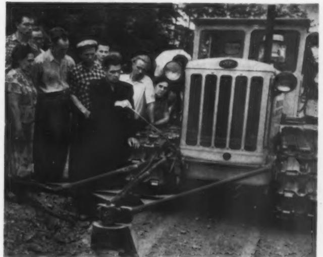
Ivan Loginov, a tractor mechanic from Kazakhstan, demonstrates an automatic tractor he invented that can operate without a driver.
