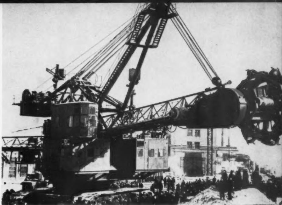
The plant makes this continuous-action rotary bucket excavator used for open-pit coal and iron ore mining.
