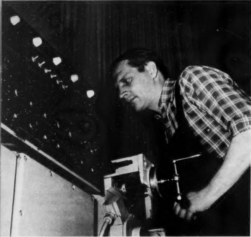
*This turret lathe machines very small parts and performs a number of operations automatically. The operator is a control command device.*
