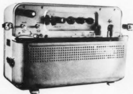
*This electrogastrograph is a boon to both doctor and patient. It eliminates the need for swallowing a rubber tube to examine the stomach. A number of electrodes are applied to the body to give the organ's biological potential.*
