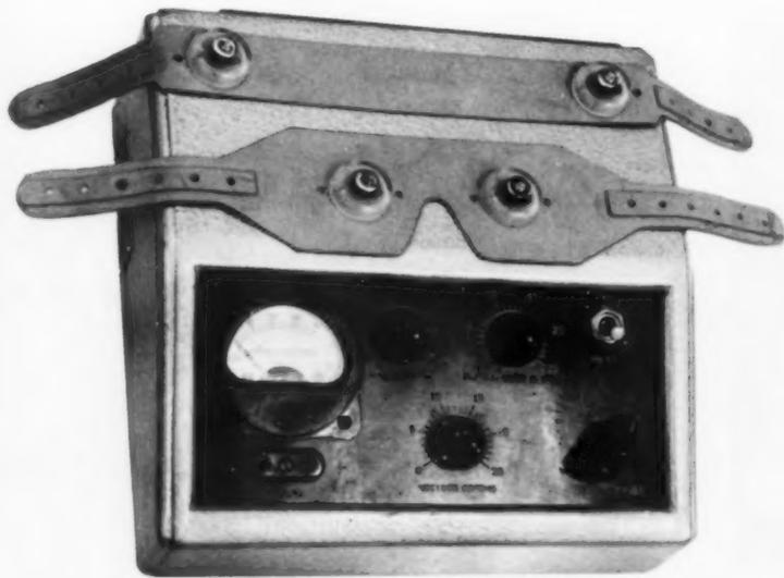
A portable "electric sleep" unit for use by surgeons, psychiatrists and therapists. Electrodes are placed on the patient's eyes and back of the head. They inhibit the nerve cells, produce a drowsy state and then sleep. In most cases the patient keeps on sleeping after the current is turned off.
