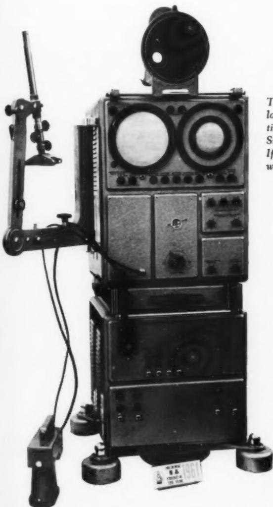
*This instrument is designed to diagnose and locate tumors and other pathological formations. It operates on the radar principle. Supersonic impulses are sent into the body. If they meet a tumor or other neoplasm on the way, the impulses are reflected on the screen.*
