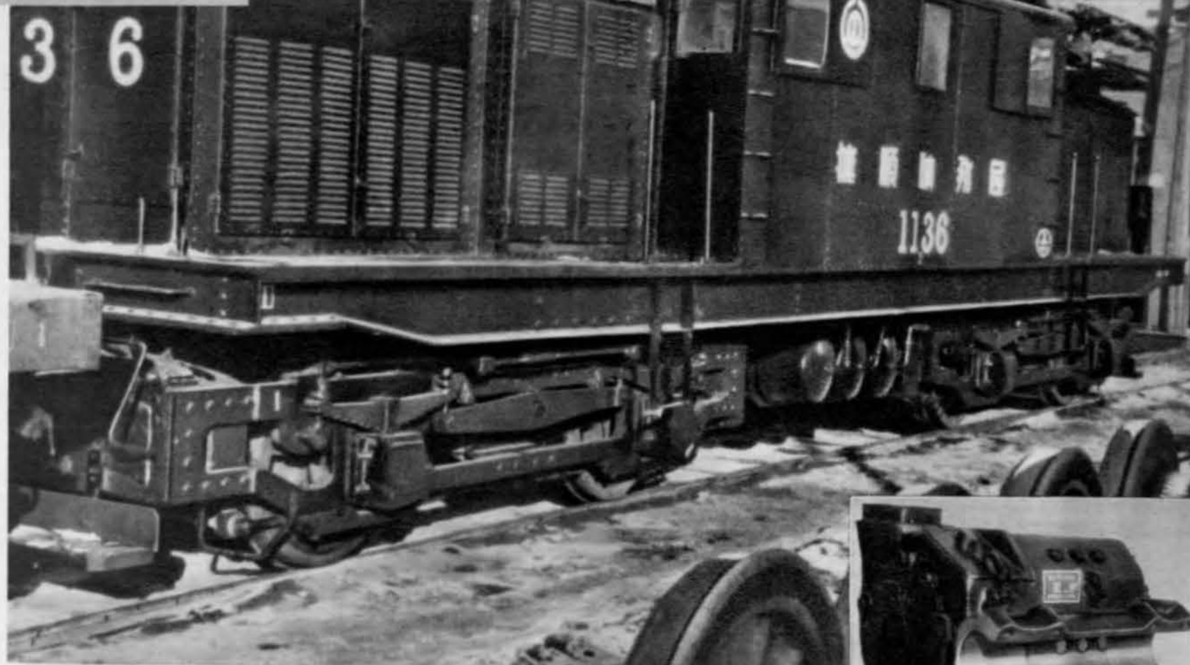
The Electric Motor Department of the Fushun Colliery manufactures a 325-H.P. D.C. electric motor—with the successful production of this powerful electric motor, derelict rolling stock has again been brought into use for the transport of coal
