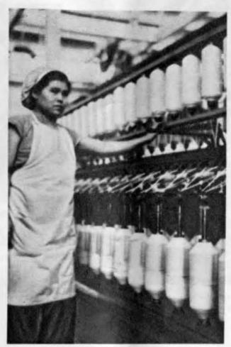
COARSE SPINNING-the rovings are set on an intermediate frame and spun
