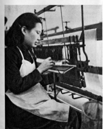
HEDDLING—the warp threads are guided through the heddle eyes to the lathe of the loom
