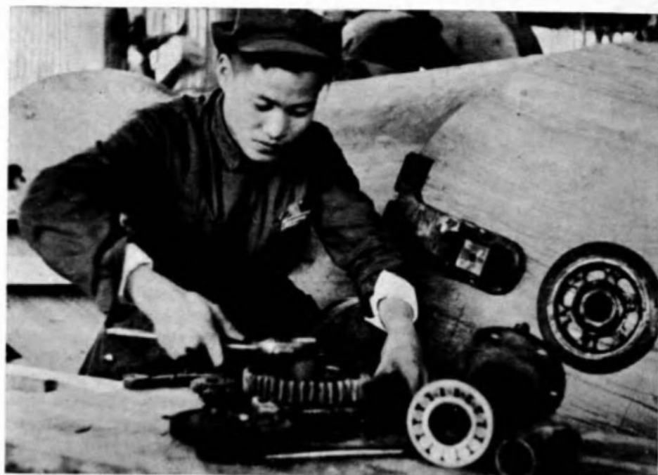
Huang Yung-chang assembling a circular saw which has been built from scrap.
