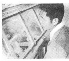
Rubber gloves attached to Jin Liangcheng's sterile inoculation boxes allow him to work inside the boxes without contaminating the fungi contents,
