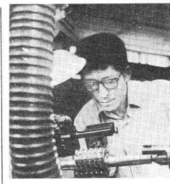
Yang Fulin works on a high-precision turbine hobbing cutter jointly developed by himself and fellow technicians of the Shanghai Implement Factory. Xinhua
