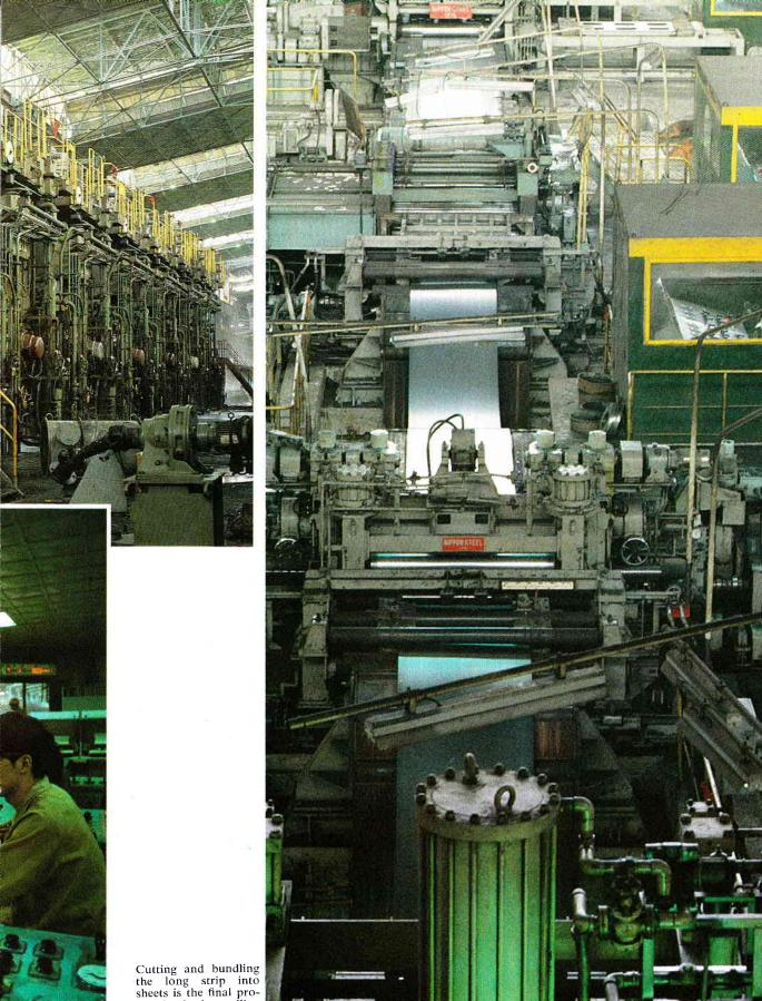
Cutting and bundling the long strip into sheets is the final pro-cess in the hot rolling mill.
