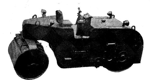
Types: Two or three-wheeled road rollers with 6-8, 8-10 or 12 ton capacity.
